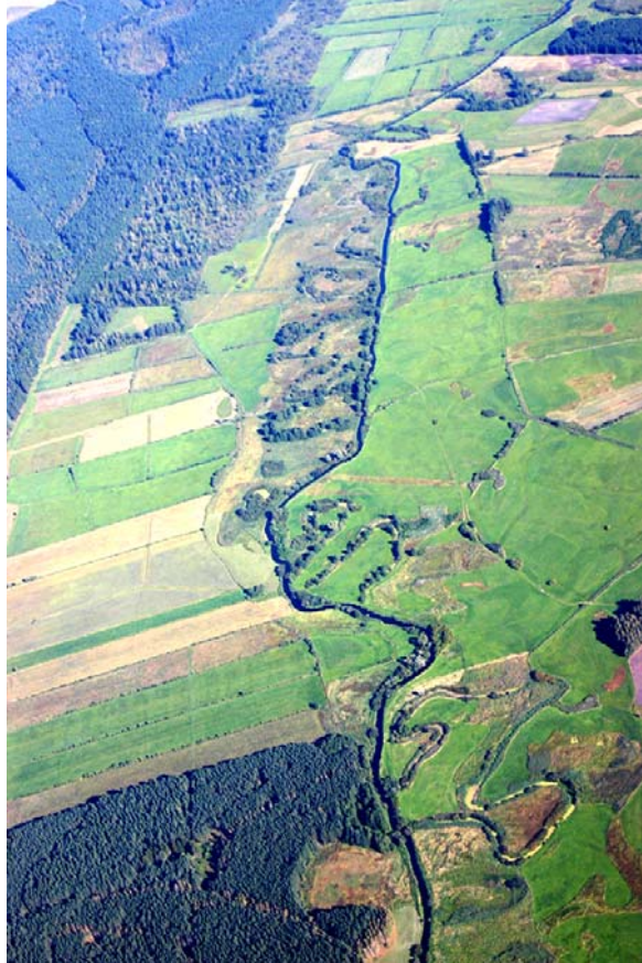
Photo 1. Fragment of the Drwęca river bed beneath Drwęckie lake straightened in 30s of the 20th century with visible cut off meanders (photo by K. Glińska-Lewczuk)
