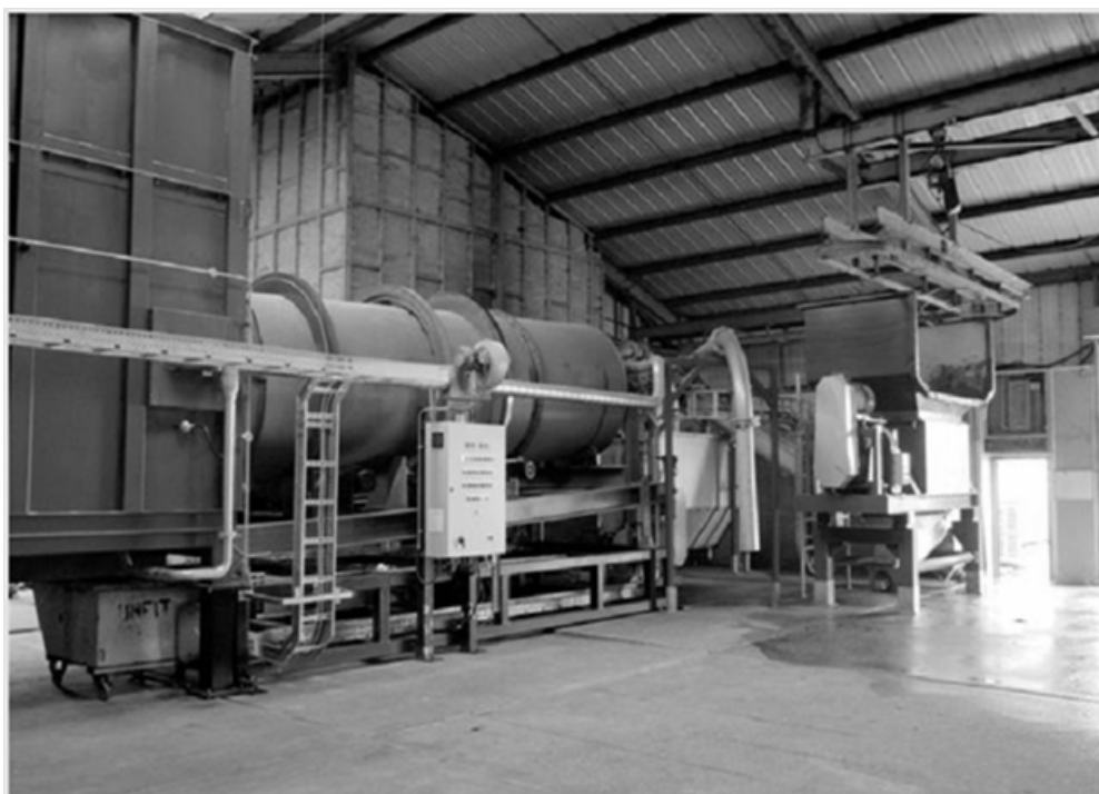
Fig. 1. Animal carcass thermal destruction system with a rotary kiln, capacity: 500 kg/hour (courtesy of Todaysure Project Ltd)
