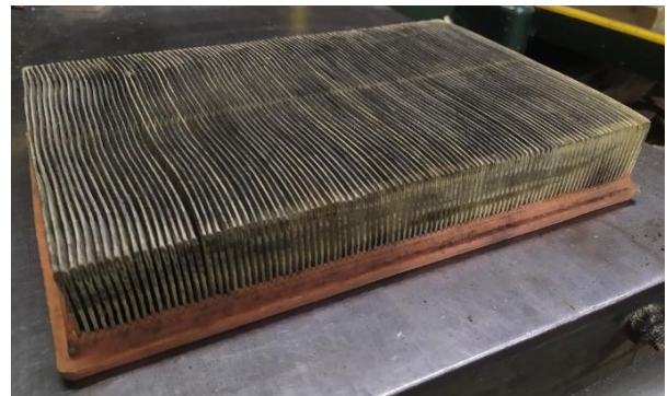
Figure 5.5. Used standard air filter with a mileage of 20,000 km
