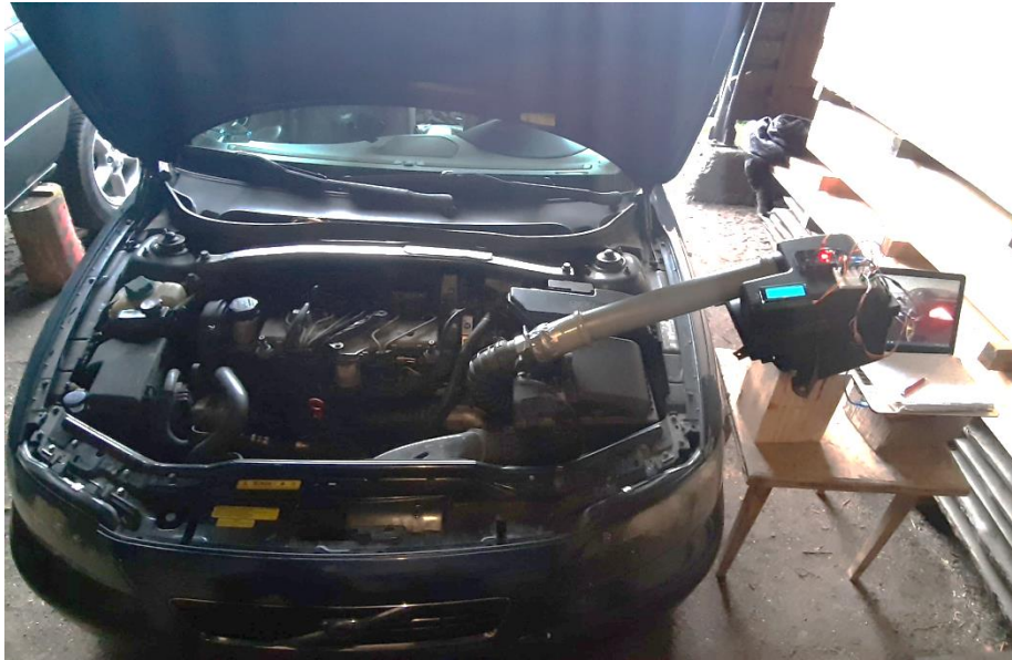
Figure 5.6. Measuring device connected to a compression ignition engine
