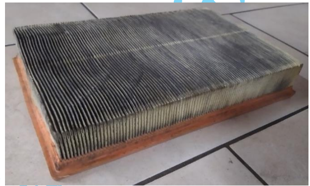
Figure 5.4. Used standard air filter with a mileage of 10,000 km
