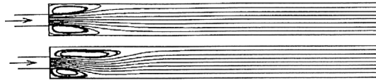
Fig. 6. Current contour lines for Re = 53 (upper) and Re = 67 (lower) Source: BATAGLIA et al. (1997).
