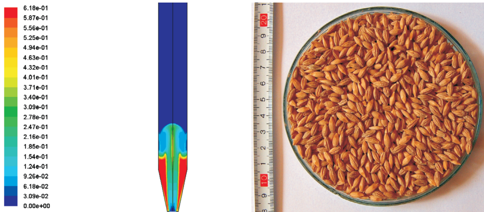
Fig. 5. Solid phase distribution in a spouted bed grain dryer
