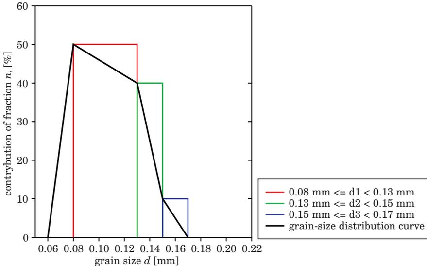
Fig. 3. The histogram of sediment grain size distribution used for calculations, acc. to parameters  $d_{50}$  and  $d_{90}$
