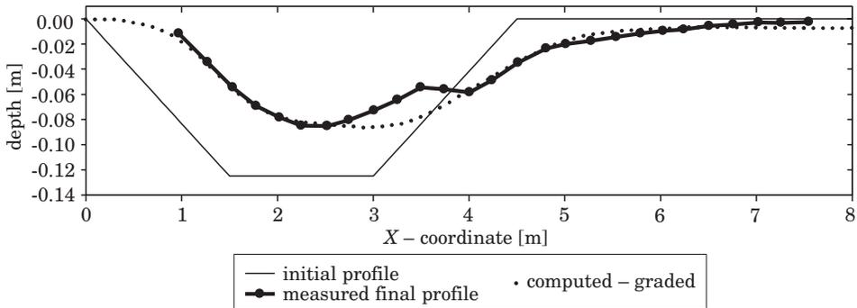
Fig. 8. Changes in the bed profile after time  $T = 10$  hrs. Comparison of the results of modelling for non-uniform sediment (including changes in the grain size distribution) with measurements
