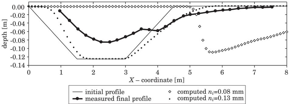
Fig. 5. Changes in the bed profile after time  $T = 10$  h. Comparison with the results of modelling for non-uniform sediment
