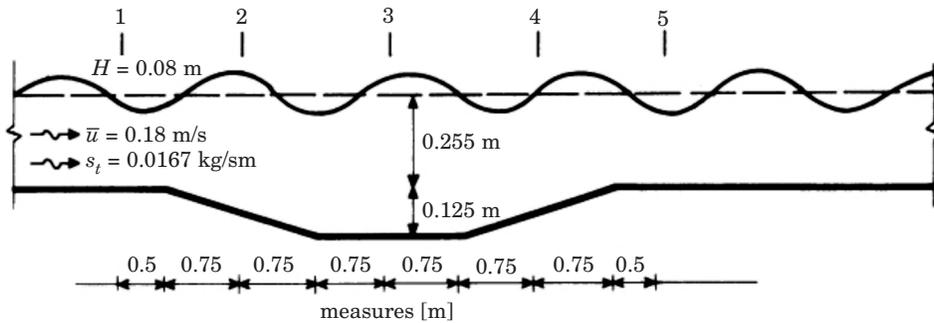
Fig. 2. Location of the measurement sites along the canal
