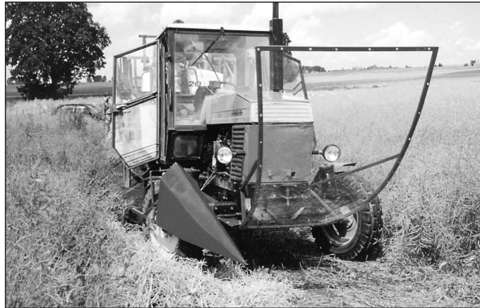
Fig. 1. Spraying unit equipped with a screen, canopy dividers and tractor undercarriage casing
