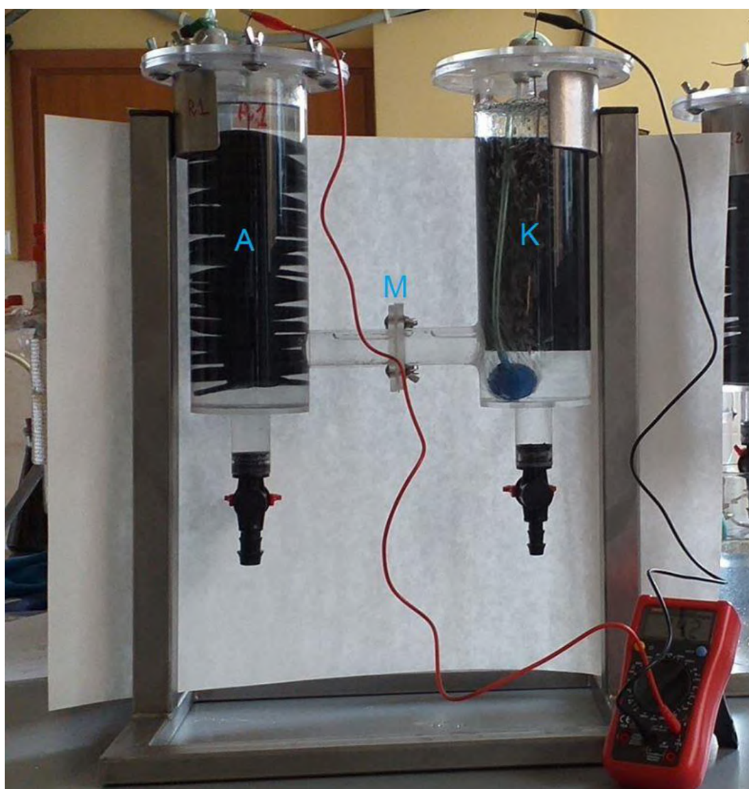
Figure 1 SM. Design of a dual-chamber MFC reactor, where A- anode chamber, K- cathode chamber and M- PEM membrane.
