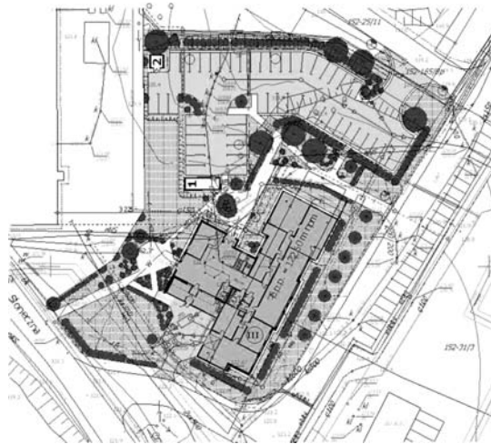
Fig. 11. The development plan for the Centre of Environmental Biotechnology UWM. Designation: III – a three-storey building of the Centre, the thin line shows the outline of the demolished fodder storehouse, 1 – a roofed bicycle stand, 2 – a trash bin. Drawing: M. DEJA
