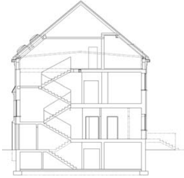
Fig. 6. A sectional view of the old building in Bydgoska Street. Visible are the existing flat roof and the new gable roof. Drawing: B. DEJA
