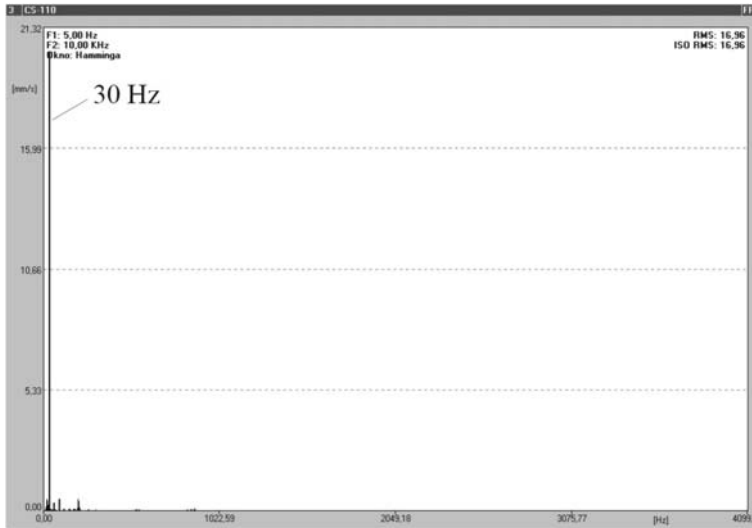
Fig. 6. A vibration speed spectrum for a centrifuge no. 1, measuring point no. 3
