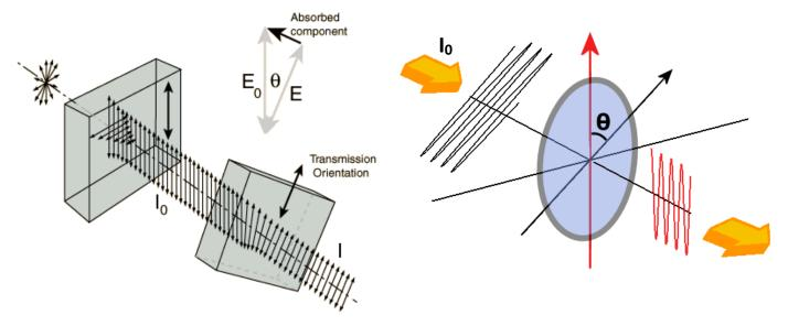
The polaroid material used in sunglasses makes use of dichroism, or selective absorption, to achieve polarization.
